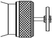
1. Pull back the draw bar of the spray gun. The material inlet is now open and both the material control needle will be cleaned.
