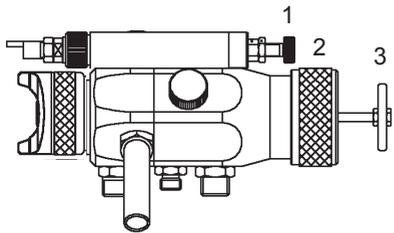
The material flow rate for the component (B) can be adjusted by turning the adjusting screw (1).
