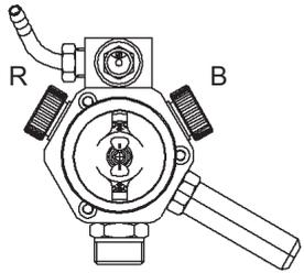
An optimum spray pattern can be adjusted by using control screws R and B. The control screw R regulates the round jet, the control screw B the wide/flat jet.
