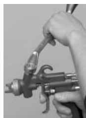
3. Use it to seal the gravity-cup material duct
