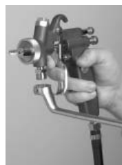
4. Screw in the double nipple and fasten.
